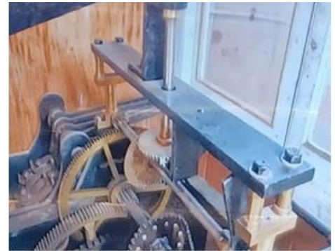
Gears and levers controlling the bells
